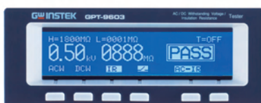
Large LCD, High Intensity Indicators and Function Keys
